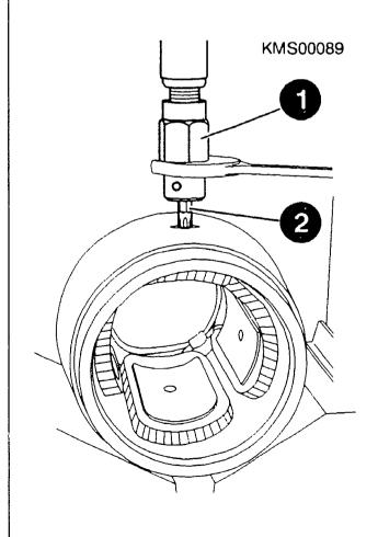
CHECKING AND REPAIRING COMPONENTS Replacing excitation winding Installation: Warm excitation windings before fitting, insert with pole shoes in stator frame and slightly tighten screws. Pay attention to markings. Press in driving-in mandrel (1). Driving-in mandrel diameter: 84,50-0,05 mm (improvisation)
